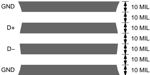
Figure 15. Arrangement of Signal Tracks
