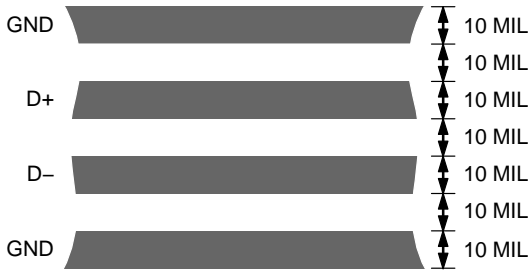
Figure 19. Arrangement of Signal Tracks
