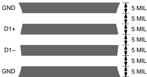
Figure 17. Arrangement of Signal Tracks
