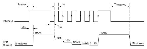
Figure 26. EN/DIM Digital Dimming Timing Diagram
