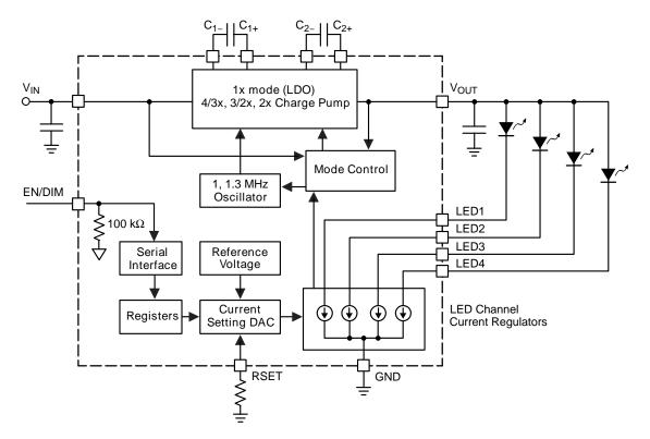
Figure 25. CAT3644 Functional Block Diagram
