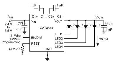
Figure 1. Typical Application Circuit
