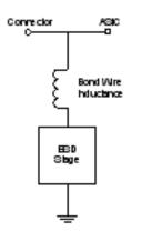
Figure 3. Standard ESD Protection Model
