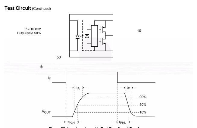
Figure 30.  $t_{PHL}$ ,  $t_{PLH}$ ,  $t_{R}$  and  $t_{F}$  Test Circuit and Waveforms
