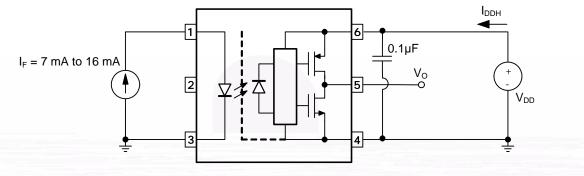
Figure 25. I<sub>DDH</sub> Test Circuit
