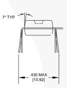
Figure 8. 8-LEAD, MDIP, JEDEC MS-001, .300-INCH WIDE
