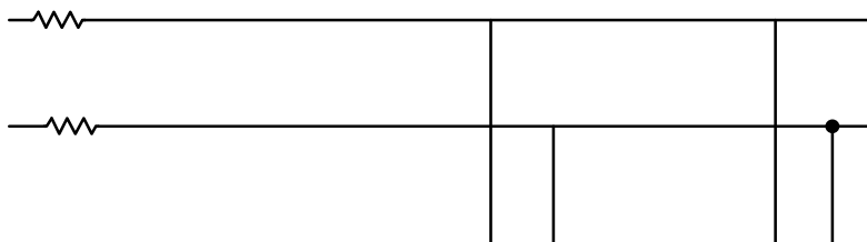
Figure 3. Typical Termination for Output Driver and Device Evaluation
