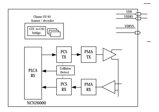
Figure 1. NCN26000 Block Diagram
