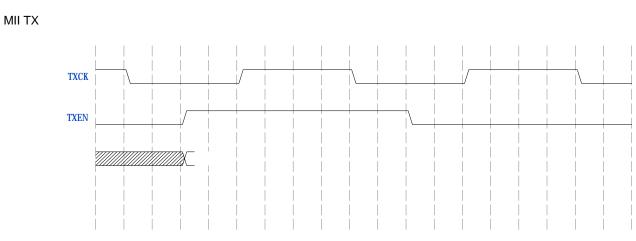
Figure 2. MII Transmit Timing
