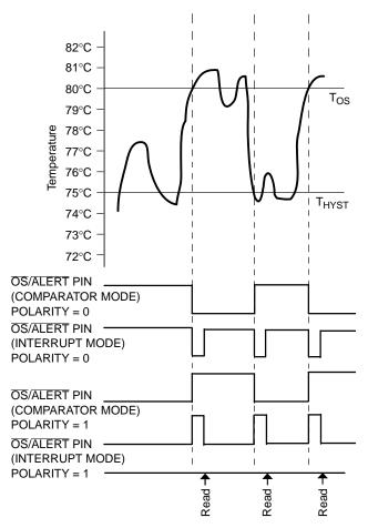
Figure 4. One-shot OS/ALERT Pin Operation
