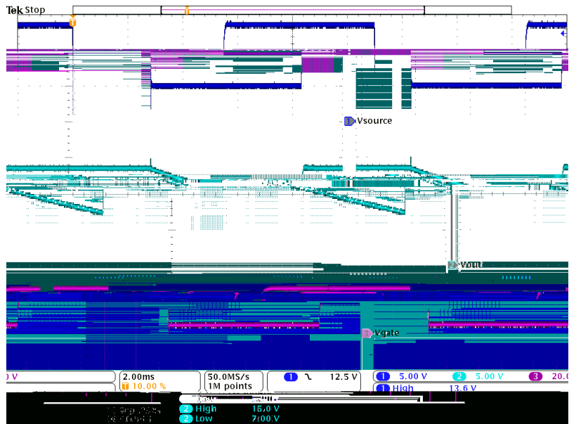
Figure 19. Application Response to Transient on the Input ( V_{Source} ) from 13.5 V to 5 V – Ideal Diode Application (see Figure 1)
