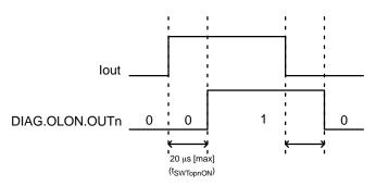
Figure 26. Direct Channel Event Delay Time
