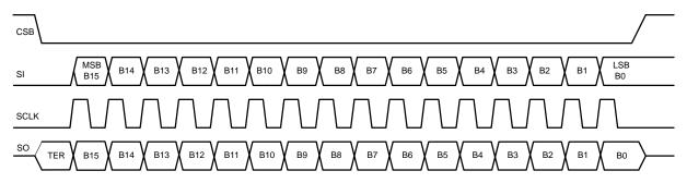
Figure 37. Serial Peripheral Interface
