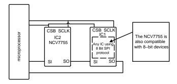
NOTE: Compatibility Note the SCLK timing requirements of the NCV7755. Data is sampled from SI on the falling edge of SCLK.
