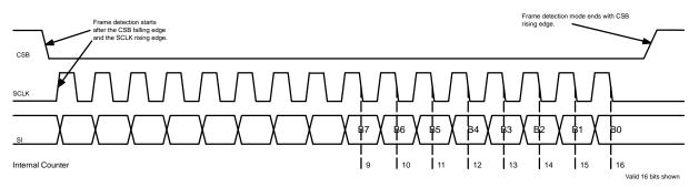
Figure 38. Frame Detection
