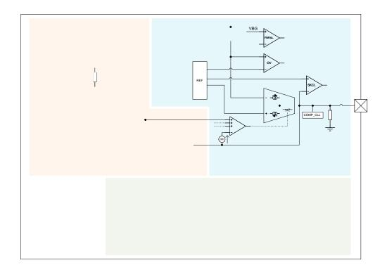
The maximum current must be set in order to allow the total desired booster power for the lowest battery voltage. Warning: setting the current limit too low may generate unwanted system behavior as uncontrolled de-rating of the LED light due to insufficient power.
