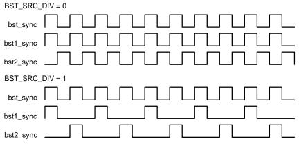
Figure 18. PWM Generator Clock Divider
