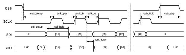
Figure 11. SPI Communication Timing
