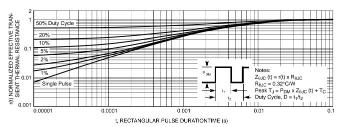
Figure 13. Junction to Case Transient Thermal Response Curve
