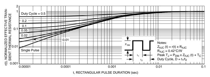
Figure 13. Junction-to-Ambient Transient Thermal Response Curve
